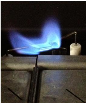
Normal Pilot Flame Pattern
