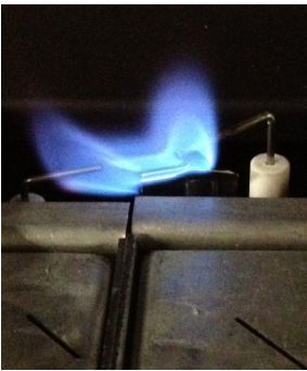
Normal Pilot Flame Pattern
