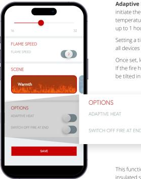
Adaptive Heat: The heater will predict and initiate the optimal time to reach your set temperature, therefore activating the heat up to 1 hour prior to the set time.\*
