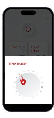
When the desired temperature button is pressed, a temperature dial will appear on screen.
