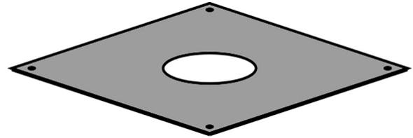
The square suspension plate is installed above the ceiling, remaining completely hidden from view. Unlike the round plate, it does not provide a visible trim, requiring additional finishing around the pipe for a polished ceiling appearance.
